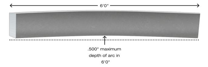
Produced to meet or exceed ASTM B505
